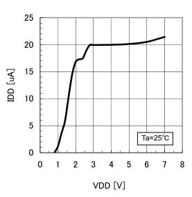
Fig2. Supply Current vs. Supply Voltage
