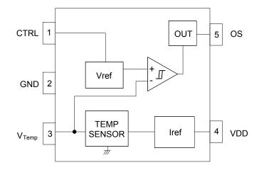
●Functional Diagram (ex. Detection Temperature 110°C)
