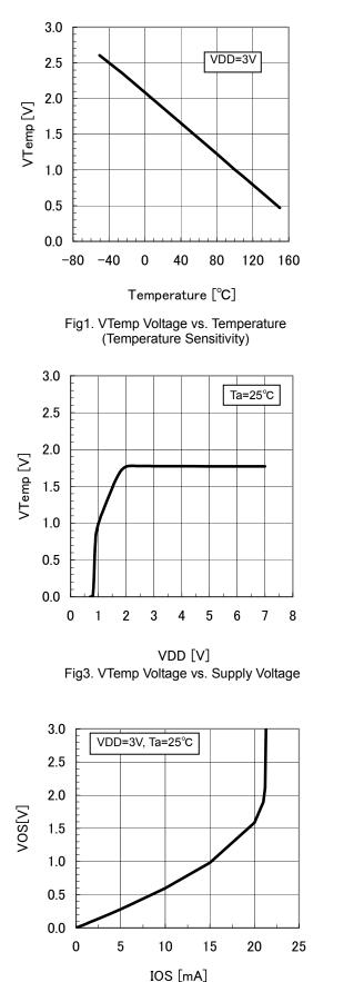
Fig5. OS Output Voltage vs. Load Current
