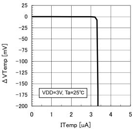
Fig4. VTemp Voltage vs. Output Current
